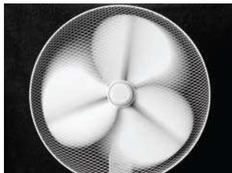
At full power here, flash duration was estimated at 1/600sec, and it got slower at lower power outputs.
