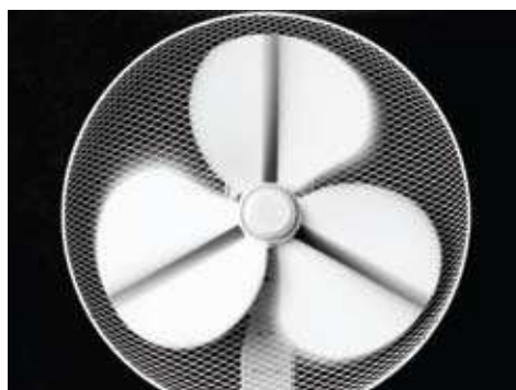
Durations can be very short at lower powers. Estimated at 1/1100sec here using the -2 stops switch.
