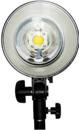
The standard flash head has an extremely bright LED modelling lamp , covered by a yellow filter (see photo on the left). This produces a powerful, consistent light at 5500K, ideal for video use as well as its primary function as a modelling lamp. It is not user replaceable but, with reasonable care, it should have a very long life. **LED modelling lamps are very cool running and are very efficient, but they do get hot if used for long periods of time.**
