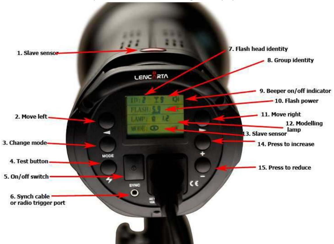
1. **Slave sensor.** This 'sees' the light from another flash and, if switched on, will trigger the flash head instantaneously. It will also operate on the infra red wavelength.
