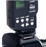
Switch the transmitter on, using the on/off switch mounted to the left hand facing side of the transmitter unit.
