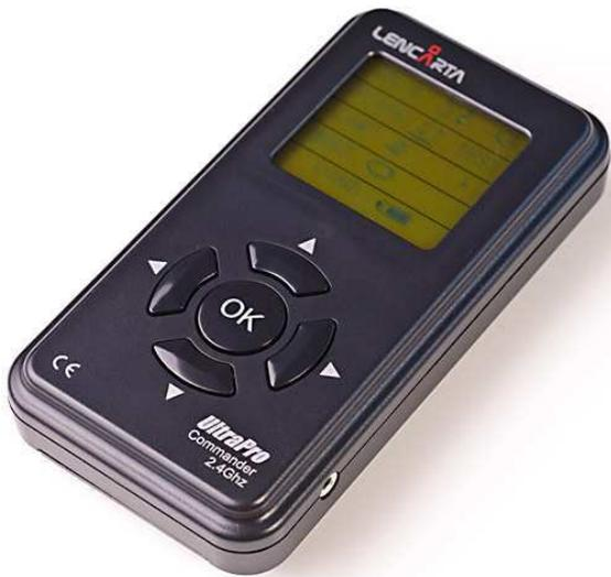
The Commander is a fully featured remote control. It can control all functions of our UltraPro flash heads, and can also control up to 10 flash heads in up to 10 separate groups, at a distance of up to 100 metres.
