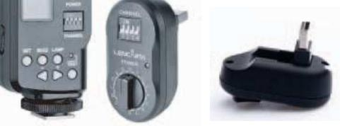
The transmitter slides into the camera hotshoe, with the controls facing the rear of the camera. It will work with any type of hotshoe except for the proprietary Sony/Minolta hotshoes, for which an adapter is needed. Once fitted, the knurled locking wheel should be gently tightened. Please note that over-tightening can damage the unit, and can also prevent reliable operation.
