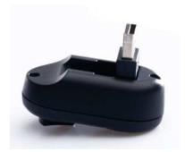
The transmitter slides into the camera hotshoe, with the controls facing the rear of the camera. It will work with any type of hotshoe except for the proprietary Sony/Minolta hotshoes, for which an adapter is needed. Once fitted, the knurled locking wheel should be gently tightened. Please note that over-tightening can damage the unit, and can also prevent reliable operation.
